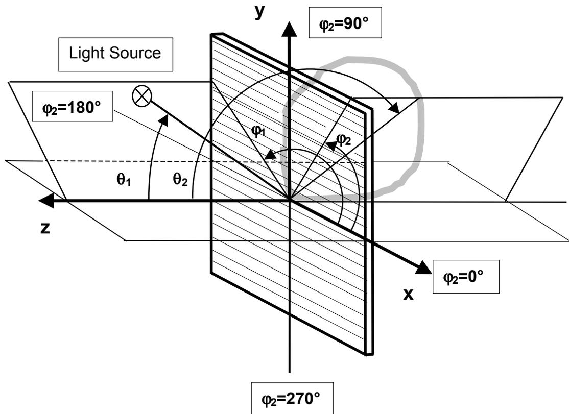
Fig. 3: Co-ordinate system for material measurements
