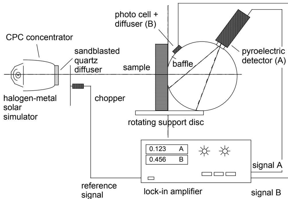
Fig. 4: Principle of the monitoring system
