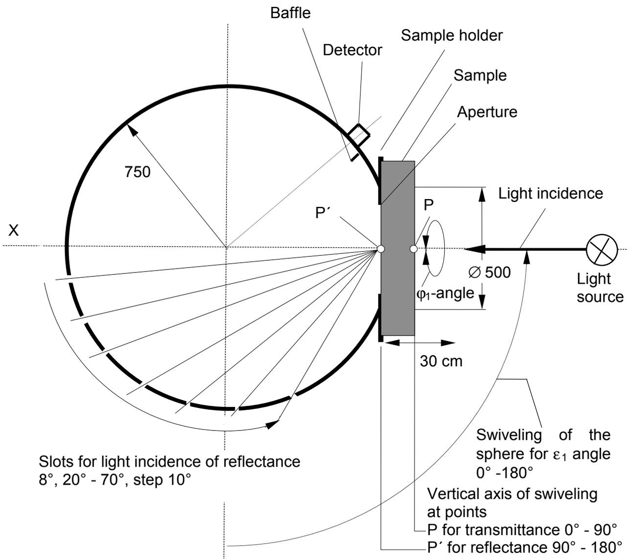
Fig. 5: Top view of the integrating sphere
