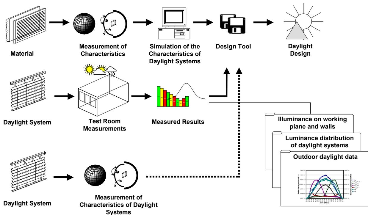
Fig. 1: The three methods for daylighting simulation
