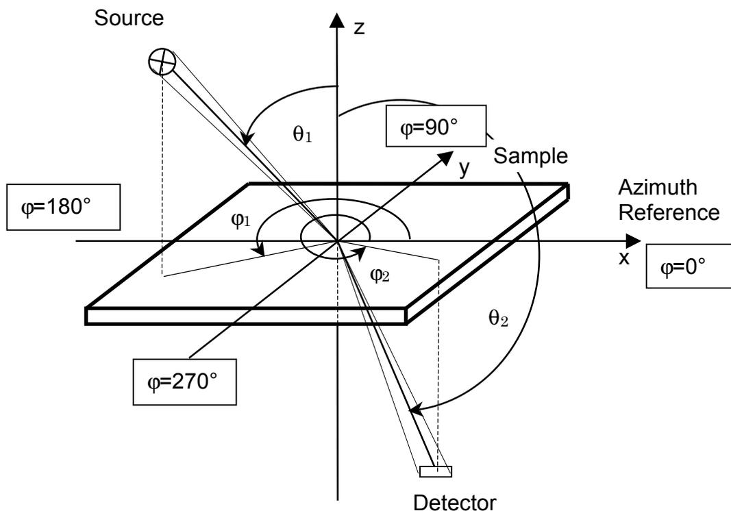
Fig. 2 : Angle notation for photometric properties
