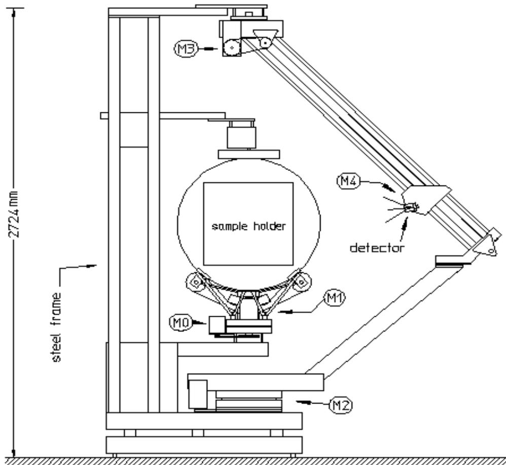
Fig. 19: Schematic side view of the sample holder and detector. M0 to M4 are the stepping motors
