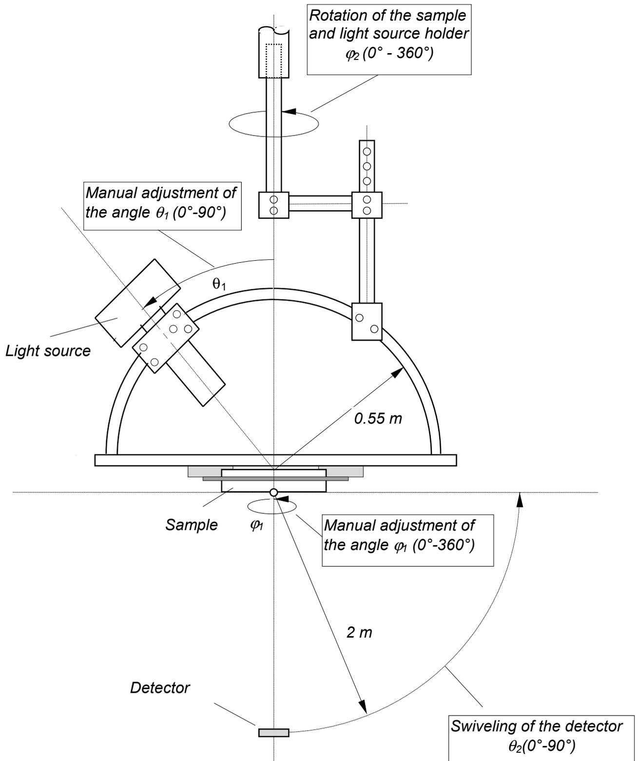
Fig. 20: Side view of the spiral goniophotometer
