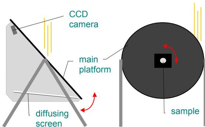
Fig. 16: Rotation of main platform and sample holder
