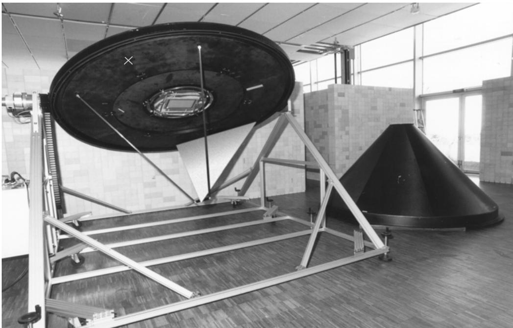
Fig. 15: Bi-directional Goniophotometer developed at LESO-PB/EPFL. The CCD camera (absent on the picture) is fixed on the rotating ring at the cross mark.
